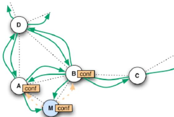
Fig 3 First nodes (A, B) get the update from node M.
